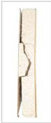
Rigid plastic wall panel - complete structural failure.
